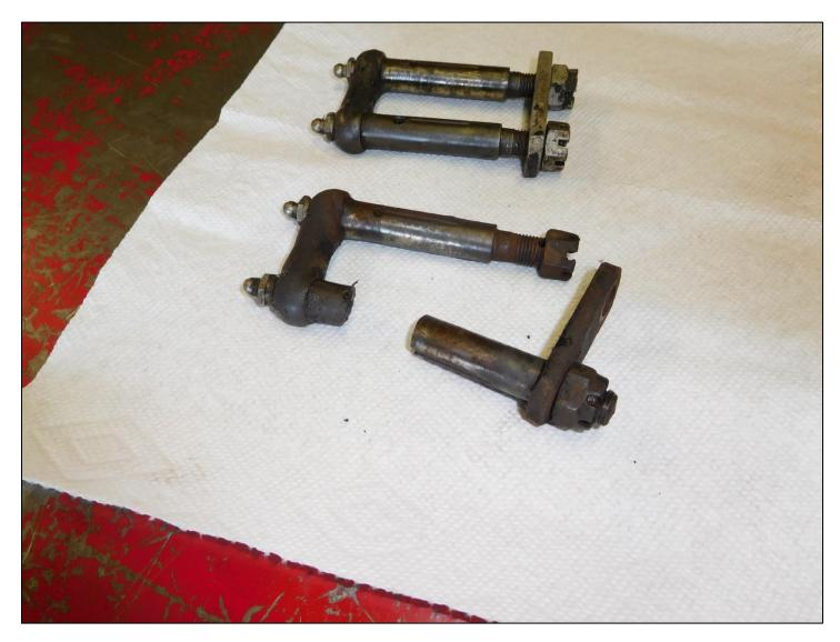
The left rear shackle was found broken while removing the rear axle assembly from my grandson's 1930 Tudor during restoration. This is why it is never a good idea to pull the rear end with the spring attached to it. The rear spring could have broken loose and flown in any direction once the spring was free from the frame.
