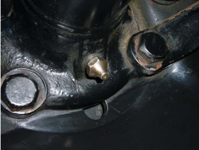
Grease fitting located on the rear axle housing
