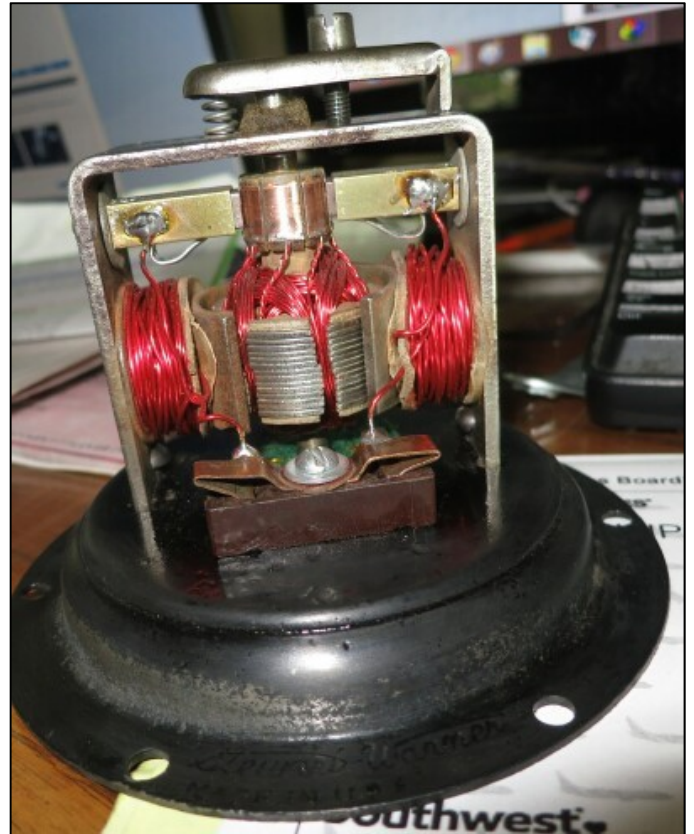
Rewound field and armature by Steve Smith
